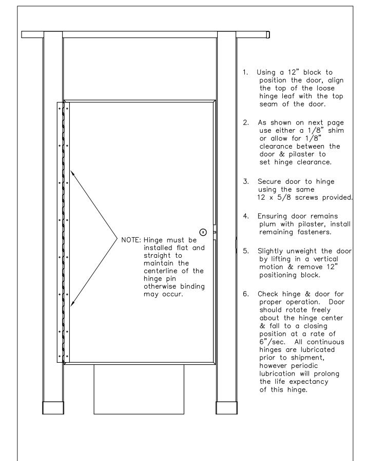
HADRIAN recommends the use of a LPS II Lubricant as a regular maintenance procedure. Although any Industrial type non—drying lubricant which has been formulated to leave a light oily film will provide adequate protection against corrosion & premature wear.
